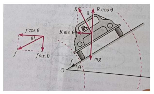
R is broken into  $Rsin\theta$  which provides requisite centripetal force &  $Rcos\theta$  which balances the weight of the vehicle.
